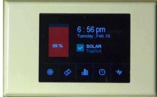
If the tank reads "0%" then there might still be 1/3 hot water remaining (depending on temperature of that upper 1/3). This is your reserve and controller action is most likely needed to maintain the supply of hot water, useful in avoiding cold showers.
